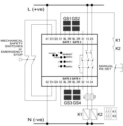
**CONTROL CONTACTS**: Two sets of positively guided N/O safety contacts on terminals, 13,14; and 23,24 (rating 4 Amps). One auxiliary N/C contact, (31-32). External fusing is recommended.
