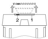
The central part of the ISIS control unit lid (1) is removable. Using a small screwdriver in the recess (2) gently prise the lid upwards. This allows access to the Automatic/Manual monitored Reset switch and the Guard Selector Switch.
