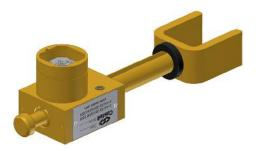
The KC Lock is a key operated mechanical bolt interlock suitable for the control of electrical switchgear. The standard unit comes with a 16 mm diameter bolt fitted with a claw, that is used to control the rotation or movement of the operating handles or toggles of electrical switchgear. The bolt length and claw dimensions are variable to suit the particular requirement. The lock is manufactured in brass or stainless steel making it ideal for use in harsh or corrosive environments.
